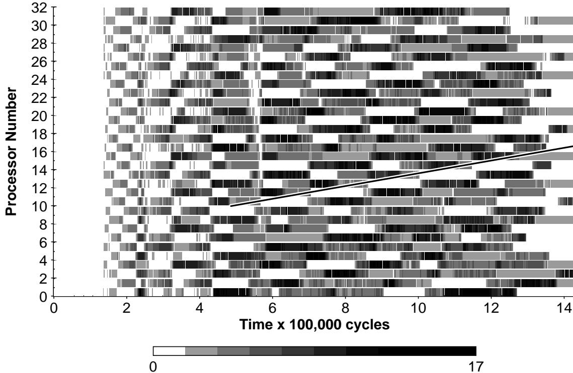
Figure 4: The total number of packets in the network headed to any given processor at any given time. Time is measured in 33-megahertz clock cycles.
