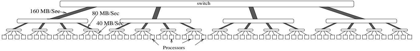
Figure 1: A 64-node CM-5 data-network fat-tree showing all of the major arms and their bandwidths (in each direction). One needs to cut only a single major arm to find the worst bisection for a given message pattern.
